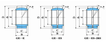
SDTZ Spherical Plain Bearings are manufactured with a single split in the outer ring in the axial direction. Both the inner and outer are phosphate treated. Sliding surfaces are steel and teflon lined.
